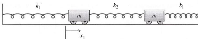
Fig. 3: Coupled Oscillation of two carts with three springs. Note the spring in the middle is different from those on the two sides and the two carts are of the same mass.
