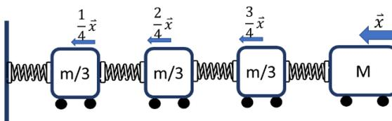
Fig. 1: The cart of mass  $M$  is attached to a spring of mass  $m$ . The spring is divided into three parts of the same mass with their speed shown above. In the question, you should divide the spring into  $n$  parts with the limit  $n \rightarrow \infty$ , where the speed of the part of the spring nearest to the cart is approximately  $\dot{x}$ .
