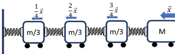
Fig. 1: The cart of mass  $M$  is attached to a spring of mass  $m$ . The spring is divided into three parts of the same mass with their speed shown above. In the question, you should divide the spring into  $n$  parts with the limit  $n \rightarrow \infty$ , where the speed of the part of the spring nearest to the cart is approximately  $\dot{x}$ .
