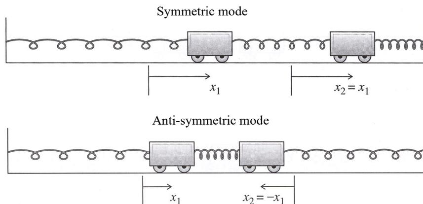
Fig. 4: Normal modes of two-cart coupled oscillation. The upper picture shows the symmetric mode where two carts move to the right by the same distance  $x_1 = x_2$ , and the lower one shows the anti-symmetric mode in which one cart move to the right by the distance  $x_1$  while the other moves to the left by the same distance.
